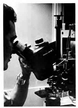
SPECIALIZED ASSEMBLY EQUIPMENT is used in fabricating hybrid microcircuits. Eliseo Chavez (2432) uses the system shown here for precise placement and bonding of active semiconductor devices on hybrid circuits.
